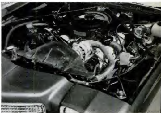
BIG 455 V8 is only engine available, gets lousy gas mileage. Note dead space ahead of powerplant
